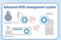
The scope reprocessing information includes the operator ID, the cycle date/time, and the machine serial number.
